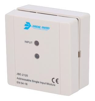
Jade Bird analog module - 1 Supervised input - Powered by loop - Conductor cable up to 2.5mm2 - REOL of 10 k? (supplied) - Certified EN 54-18
