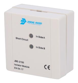
Jade Bird analog module - Short-circuit insulator - Powered by loop - Conductor cable up to 2.5mm2 - Max 32 devices per segment - Certified EN 54-17
