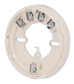
Jade Bird connection base - Basis of 4 terminals - Connection without polarity - 4 terminals, 2 loop and 2 external power supply. - Compatible with all Jade Bird devices - Allows connection of remote indicators or pilots
