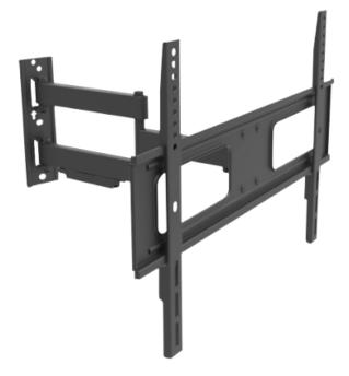
Bracket for LCD monitor - Wall installation - 30° Inclination 180° Rotation - Wall separation 60~473 mm - Maximum load 50 Kg - Screens 37"~70"
