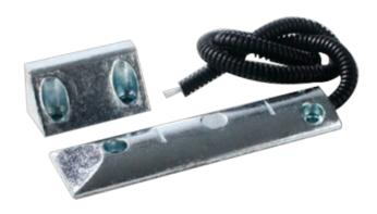
FDP magnetic contact for shutter - For installation in metal - Reed technology High power - System of 4 armored wires - Metal cover - Suitable for exterior IP65 - Grade 2 approved
