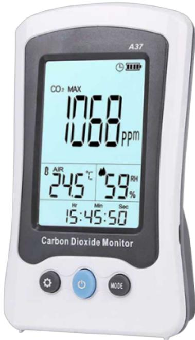
Temperature and humidity meter from CO2, - With user-programmable visual and audible alarm
