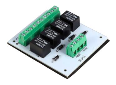
Relay module - Creation of two-door locks - Double output - Small size - For all types of doors - Power supply 12 VDC
