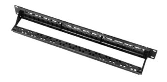
Patch blind panel from 24 ports UTP/RJ45 - Rackable format 1U - Without electronics - Size 1U for easy installation - Dual IDC: 110 IDC and Krone IDC - Includes cable organizer
