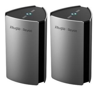
Reyee Pack 2 Router Gigabit Mesh Wi-Fi 6 AX3200 - 4 Ports RJ45 10/100/1000 Mbps - 802.11ax 4x4 dual-band 2.4 and 5 GHz - Remote Management through Cloud and App - Parental Control, Guest Network, Roaming - Designed to create a complete Mesh network
