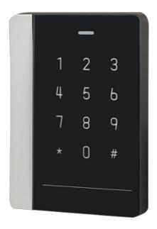
Access reader - Access by MF card and PIN - LED and acoustic indicator - Wiegand 26/34 | RS485 - Compatible with Safire - Valid for interior
