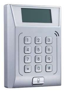
Access control - EM card and PIN - 3.000 users | 10.000 records - TCP/IP and relay - Integrated controller - Safire Control Center-software
