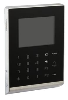
Access and Attendance control - EM card and keypad - 100.000 users / 300.000 registers - TCP/IP, USB, WiFi, Wiegand and Relay - Integrated controller - Safire Control Center-software
