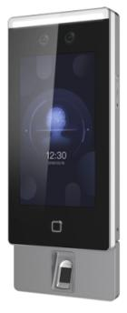
Access and Attendance control - Face, fingerprint and MF card recognition - 6.000 faces, 5.000 fingerprints/cards and 10.000 records - TCP/IP, USB and WiFi - Integrated controller (door sensor, polisher and relay) - Software Safire Control Center AC
