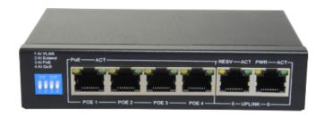
PoE Switch - 4 PoE port(s) + 2 Up-link port(s) - Speed up to 1000 Mbps on all ports - Up to 60W in total for all ports - Bandwidth 12 Gbps - Standard IEEE802.3af (PoE) / at (PoE+)
