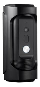
Video intercom IP - Camera 2 Mpx with pinhole lens - Bidirectional audio - Mobile App with or without monitor - Vandal-resistant zinc alloy IK09 - Surface mount : PoE standard
