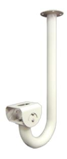
Ceiling bracket for casings - Compatible with HS250W - 470 (H) x 85 (W) x 240 (D) - Maximum load 15 Kg - Aluminum / Ivory colour - Horizontal  $360^{\circ}$  / vertical  $85^{\circ}$  rotation
