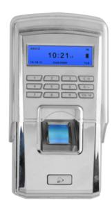
ANVIZ autonomous biometric reader - Fingerprint and Username/Password - 1000 recordings / 50000 records - TCP/IP, RS485, miniUSB, Wiegand 26 - Integrated controller - Cover for exterior use
