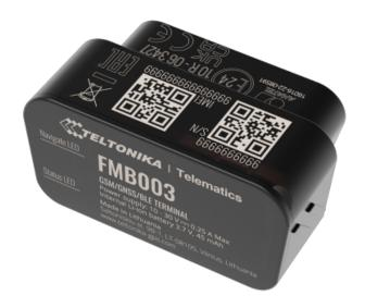
Plug & Play Tracker for vehicles - OBD connection - Fast and accessible installation - 2G and BLE for TK-EYE - Nano-SIM - OEM parameter reading
