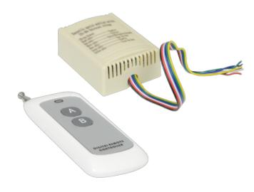
Wireless relay with control for turnstiles - 2 relays | NO / COM operation - Frequency 433 MHz - Measurements 55 x 75 x 25 mm - Cable included - Easy installation
