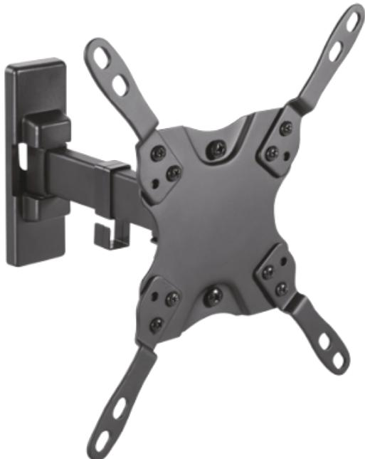
Wall bracket for LCD monitor - Inclination -12°~ 5° - Rotation -90°~ 90° - Wall separation 60~190 mm - Maximum load 20 Kg - Screens 13"~42"
