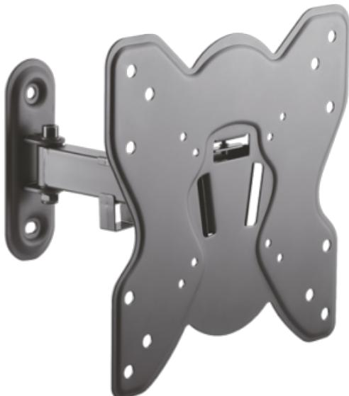
Wall bracket for LCD monitor - Inclination -12°~ 3° - Rotation -90°~ 90° - Wall separation 65~200 mm - Maximum load 25 Kg - Screens 23"~42"
