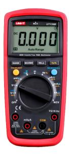
Digital multimeter with True RMS function - DC and AC voltage measurement up to 600V - DC and AC current measurement up to 10A - Resistance, Capacitance and Frequency Measurement - Buzzer for continuity test
