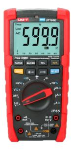
True RMS industrial digital multimeter - IP65 and 2 m drop proof - DC and AC measurement up to 1000V / 20A - Integrated flashlight - Resistance, Capacitance and Frequency Measurement - Buzzer for continuity test
