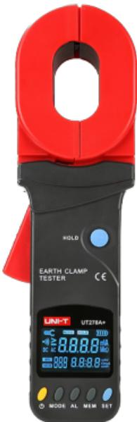
Earth fault current clamp meter - EBTN display up to 1000 accounts - Measurement of leakage current up to 30A - Earth resistance measurement up to 1000? - Auto calibration | Auto range - Resistance limit alarm
