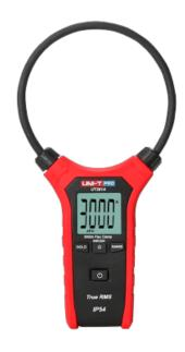
Flexible current clamp 10" - LCD display of up to 3000 counts - Current measurement in AC up to 3000A - High AC accuracy with True RMS function - Degree of protection IP54 | 2m drop test [%VAR%] - Automatic shutdown
