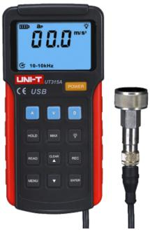
Vibration meter - Measures Accelerations, Speeds and Displacements - Use in rotating and reciprocating machinery - Display of 2000
