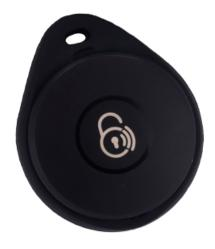
Bluetooth remote button - Bluetooth 4.2 BLE connection - Opening and closing - Compatible with WM-BOLT - Suitable for exterior IP67 - Powered by 1 x CR2032 3V button cell(s)
