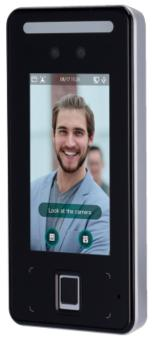
Access and Attendance control - Facial, fingerprint, keypad and MF card - 6.000 users / 150.000 registers - TCP/IP, USB, RS485 and Wiegand - Built-in controller : Suitable for outdoor use IP65 - SmartPSS Software
