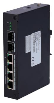
X-Security PoE Switch - 3 FE ports + 1GE + 2 GE SFP - 60W port 4 / 30W port 1-3/ Maximum 120W - Hi-PoE / IEEE802.3at (PoE+) / af (PoE) - DIN rail mount - VLAN/STP/SNMP/Loop Detection
