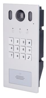
IP Video Intercom for villa - Camera 2Mpx - Bidirectional audio - Mobile App for remote monitoring - Access by code or MF card - Powered via standard PoE
