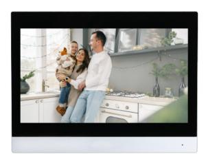
Video door entry monitor - 10" TFT Screen - Bidirectional audio - TCP/IP, WiFi and SIP - MicroSD card slot up to 64 GB - Surface mounted : Black
