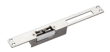
Electrical door openers - For single doors - Opening mode Fail Secure (NO) | Gate signal - Holding force 500 kg - Power supply DC 12V - Recessed mounting | Socket
