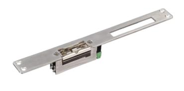
Electrical door openers - For single door | Adjustable latch - Opening mode Fail Secure (NO) | Gate signal - Holding force 300 kg - Power supply DC 12V - Recessed mounting | Socket
