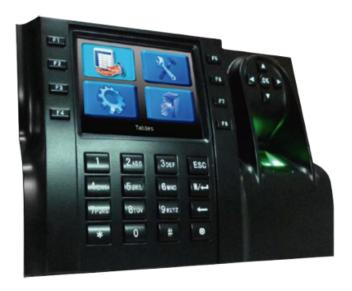
Time & Attendance control - Fingerprint, EM and MF cards and PINs - 8.000 fingerprints | 200.000 records - TCP/IP and USB - Function buttons for time & attendance - ZKBioTime software 8.2 devices included
