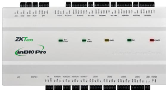
Biometric access control panel - Access by fingerprint, card or password - TCP/IP communication | RS485 - 4 Wiegand inputs | 1 input RS485 - Relay output for four doors - ZKBio CVSecurity Software
