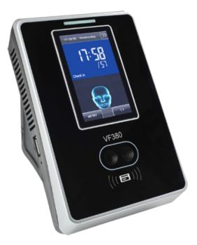
Time & Attendance and Access control - Biometric dual sensor facial recognition - Face recognition, card & PIN - 1.200 faces and 100.000 logs - 9 Modes of Time & Attendance | Integrated controller - ZKBioTime software 8 2 devices included
