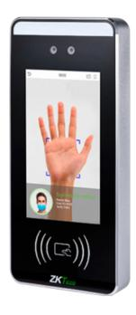
Access Control and Time & Attendance - Facial, palm, EM/MF card and PIN - 6.000 faces | 200.000 records - 5" TFT touch screen - TCP/IP and WiFi - Compatible with ZKTeco softwares
