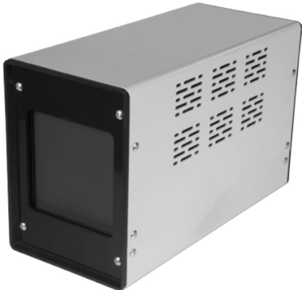
Blackbody - Calibration device for thermographic cameras - Infrared emission of 35°C ~ 60°C - Stability  $\pm 0.1\text{--}0.2^\circ\text{C/h}$  - Emissivity  $0.97 \pm 0.02$  - Guarantees a measurement accuracy of  $\pm 0.3^\circ\text{C}$
