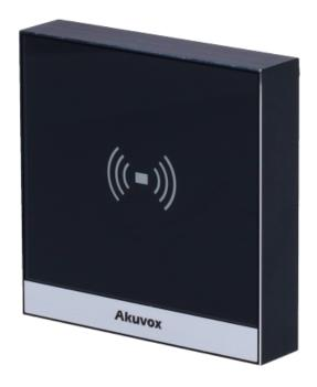
Access control - EM/MF card and NFC | 1 relay - 20.000 users | 100.000 records - Integrated controller | Wiegand 26/34 - Suitable for outdoor IP65 | TCP/IP and PoE - Connection via Cloud | Output 12V
