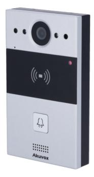
Vandal-resistant surface IP video door entry system - 2 Mpx Camera | Crystal Clear Two-way Audio - Opening with EM/MF and NFC card and 2 relays - PoE, SIP Standard - Cloud Maintenance - Connection via Cloud | Output 12V
