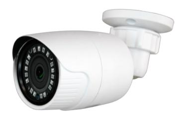
720p ECO Bullet Camera - 4 in 1 (HDTVI / HDCVI / AHD / CVBS) - 1/3" 1.3 Mpx PAS5130 - 3.6 mm Lens - 18 IR SMD LEDs Range 20 m - Weatherproof IP66
