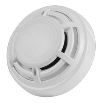
Conventional temperature increase detector - Certificate EN54 part 5 - Double LED alarm to see it from anywhere - Made of ABS material with heat resistance - Base not included - Compatible with the DMTech first version base
